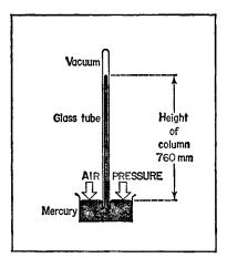
Fig. 10.1. Torricelli's experiment to illustrate the effect of air pressure.
