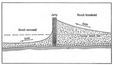
Fig. 24.2. Plan view of the effect of a groyne or jetty on longshore drift.
